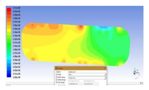
Fig. 7. Biofuels Blend Thermal NOx production rate  $Kgmol/m^3$  s
