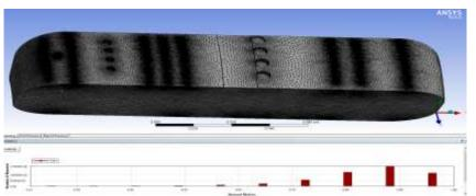
Fig. 2. Mesh generation in ANSYS MESH
