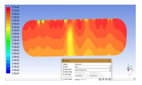
Fig. 8. JetA1 NOx production rate  $Kgmol/m^3 s$
