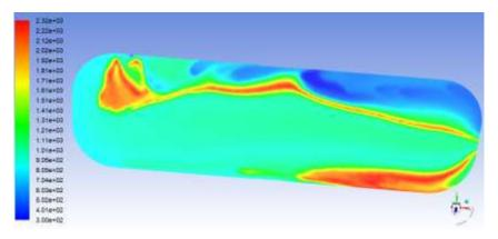
Fig. 3. Jet-A non-premixed temperature 2D contour non-premixed combustion.
