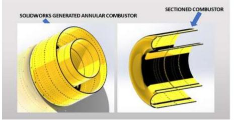
Fig. 1.: SOLIDWORKS sectioned combustor geometry
