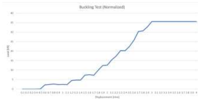
Figure 9: Load v/s displacement of normalized steel
