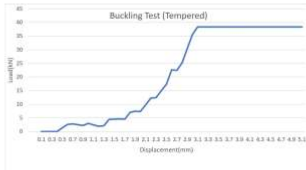
Figure 10: Load v/s displacement of tempered steel
