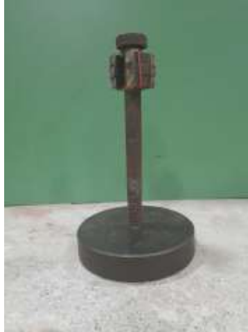
Figure 4: Modified part added in UTM
