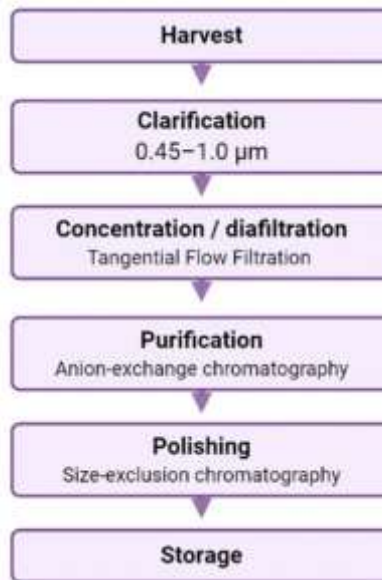
Fig 2. Flowchart for Downstream Processing of Lentiviral vectors
